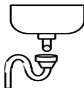
Where are air gaps required? We expect them on the 3-bay sink, dishwasher, ice machine, and prep sink. Hand wash and slop sinks do not require an air gap.
